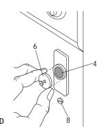
If the door has to be opened from left to right, invert the position of the plates (7), the magnet (4) and the plate (5) (Fig. B and E). Mount the countermagnet (6) and the hinges (1) as previously described.
